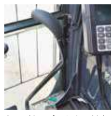
Control lever for 4-piece high reach demolition spec machine placed in the foot area
