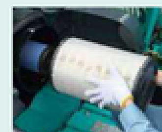
Air cleaner(double element) The double filter structure and large capacity prevents dust from being sucked in.
